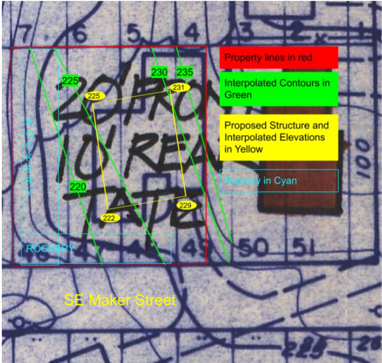
Figure 5: Interpolating Approximate Topographic Elevations of The Project based on the 1961 Survey
